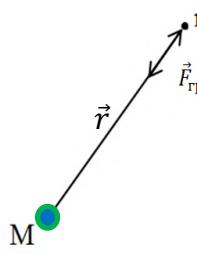
$$E_{\text{пот}}(\vec{r}) = E_{\text{пот}}(r) = \int_r^{\infty} \vec{F}_{\text{rp}} \cdot d\vec{r} = - \int_r^{\infty} G \frac{mM}{r^2} \frac{\vec{r}}{r} \cdot d\vec{r}$$
