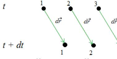
$$\delta A = \sum_{i=1}^N \delta A_i = \sum_{i=1}^N \vec{F}_i \cdot d\vec{r}_i = d\vec{r} \sum_{i=1}^N \vec{F}_i = d\vec{r} \sum_{i=1}^N \frac{d\vec{p}_i}{dt} = d\vec{r} \cdot \frac{d}{dt} \sum_{i=1}^N \vec{p}_i = d\vec{r} \cdot \frac{d\vec{p}_{\text{сист}}}{dt}.$$
